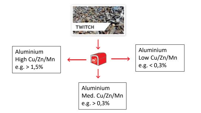
• "REDWAVE 3-step-sorting": sorting of TWITCH by content of copper, zinc and manganese in the aluminum stream
