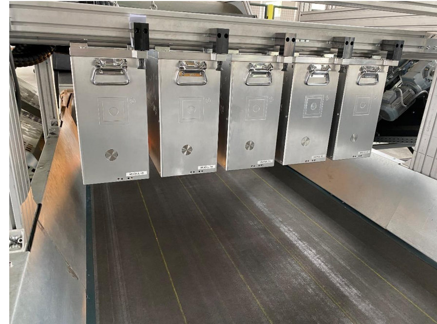
Cascade of multiple clean2sort modules to cover wide conveyor belts
