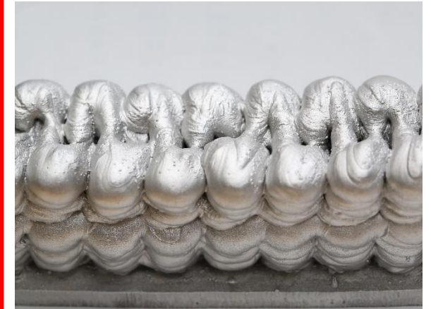
Lack of Fusion
