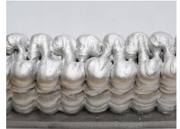
Lack of Fusion
