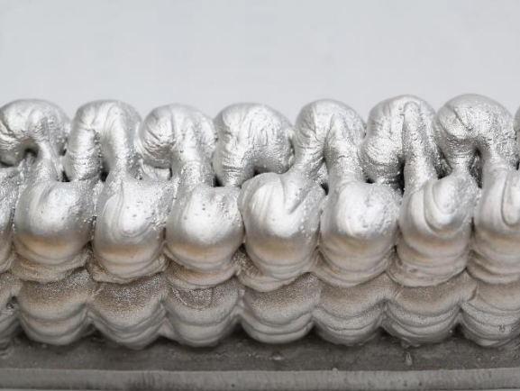
Lack of Fusion
